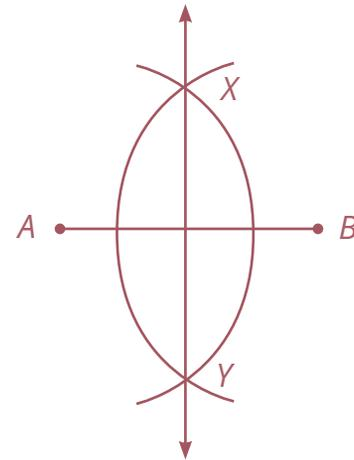
This bisector of the segment is also perpendicular to the segment at its midpoint. It is sometimes called the *perpendicular bisector* of the segment.
