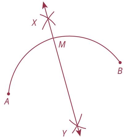
The point  $M$  where the bisector intersects the arc is called the *midpoint of the arc*. Any line, segment, or ray that passes through this midpoint is also a bisector of the arc.
