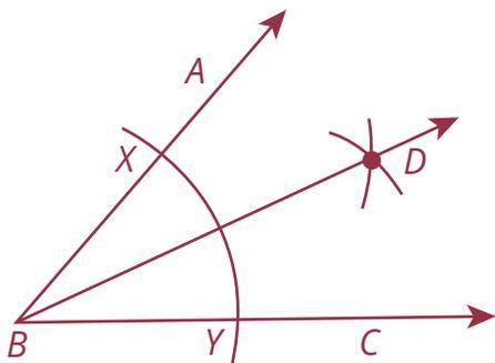
**Steps:** Using a convenient radius and the vertex of the angle  $B$  as center, construct an arc that intersects both sides of the angle. Call these points  $X$  and  $Y$  as centers and a radius greater than half of  $XY$ , construct two arcs that intersect in the interior of  $\angle ABC$ . Call this point  $D$ . Draw  $\overrightarrow{BD}$ .  $\overrightarrow{BD}$  is the ray that bisects  $\angle ABC$ .
