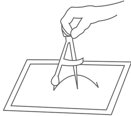
Tip the compass slightly in the direction you are drawing so that it is not perpendicular to the paper and pull the compass through your circle. Never push the compass, because pushing may tear your paper.
