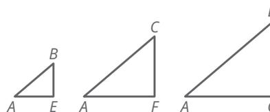
Since the ratios of corresponding sides of similar triangles are equal,  $\frac{BE}{AB} = \frac{CF}{AC} = \frac{DG}{AD}$ . For  $\angle A$ , each of these ratios represents the opposite side over the hypotenuse. For all right triangles that can be drawn with the acute  $\angle A$ , this ratio will always be the same value.
